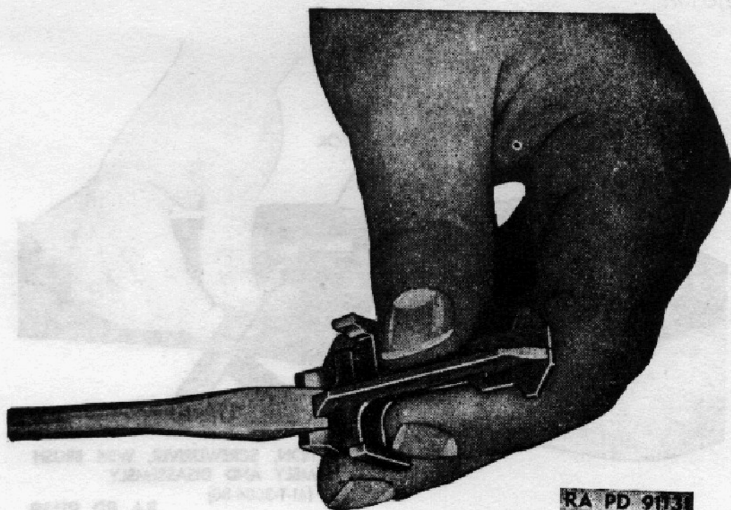
Figure 27. Removing follower slide from follower.
