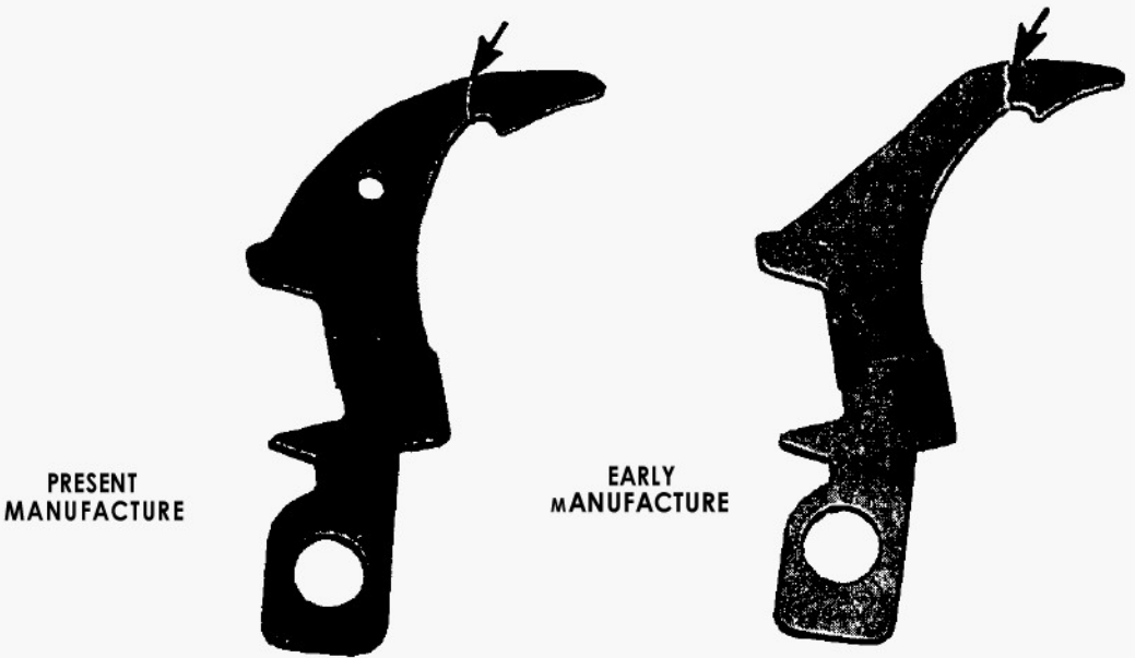
Figure 61. Points to be inspected on the hammer.
