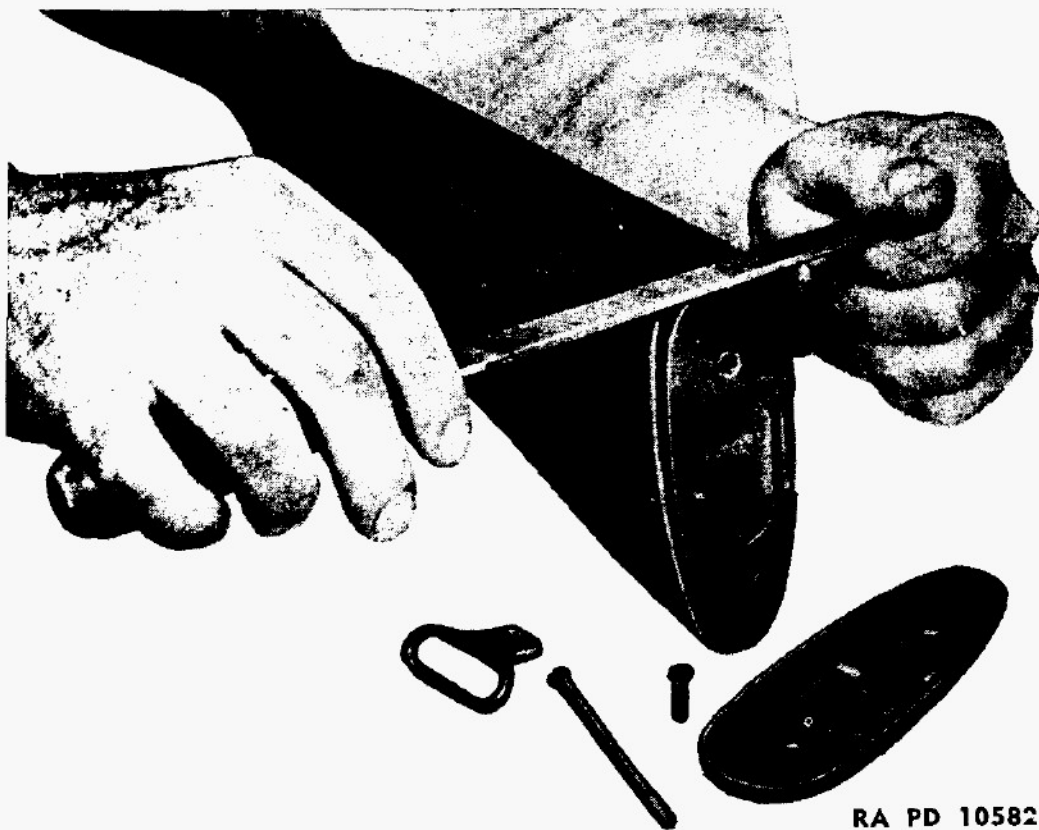
Figure 74. Fitting butt plate on stock.
